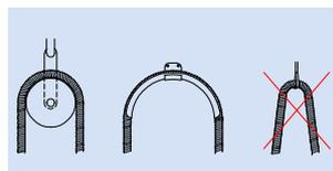
Install the hose conduit as 180 ° arc with sufficient straight ends as illustrated. Measure the installation distance according to the required bending radius.
