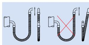
Arrange hose conduits that way that they do not come into contact with ground, walls or other objects.
