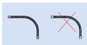
Avoid too strong bending stress by the use of a roll or a hose saddle corresponding to the allowed bending radius.
