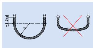
Avoid irregular distortion directly behind the connection armatures. Note the minimum bending radius.
