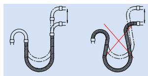
Guide motion and hose axis should lay in the same surface plane. Thus prevents any damaging torsional stress.
